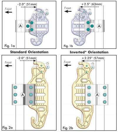
(\*Requires the mounting plate to be disassembled from the cane clamp and rotated 180°)
