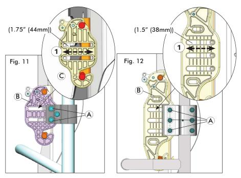
**NOTE:** The range of depth adjustment will be reduced when the angle of the Elite E2S/E2D back (mounting plate) is altered.
